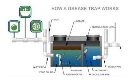
For a grease trap, or interceptor, to function properly, the FOG and solids must be removed from the trap regularly. Regular cleaning of the trap prevents FOG and solids from flowing into our sewer lines and also prolongs the working life of the trap.
